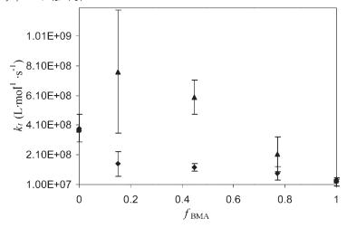
**Figure 4.** Termination rate coefficients for BMA/ST copolymerization vs BMA monomer fraction, estimated by assuming terminal propagation ( $\triangle$ ) and penultimate propagation ( $\Diamond$ ) kinetics. Error bar indicates estimated confidence intervals from parameter fitting. Homopolymerization  $k_t$  values from the literature ( $\blacksquare$ ) are also shown.
