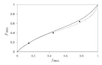
Figure 3. BMA polymer composition vs monomer composition in the semibatch reactions at 138 °C: experiment ( $\blacksquare$ ); Mayo-Lewis model (—); Lowry Case 1 model with [M]<sub>tot</sub> = 0.5 mol/L (- - -).
