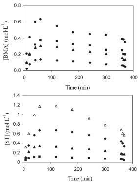
**Figure 1.**Butyl methacrylate (top) and styrene (bottom) concentration profiles for semibatch experiments of: ST homopolymerization (△); BMA homopolymerization (●); BMA/ST 75/25 copolymerization (■); BMA/ST 50/50 copolymerization (▲); BMA/ST 25/75 copolymerization (◆).
