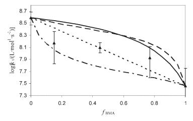
**Figure 6.**Termination rate coefficients for BMA/ST copolymerization vs BMA monomer fraction at 138 °C: estimated values (♠); Walling equation (—); Atherton and North model (— —); Buback simplified model (- - -); Ma model (— - —).
