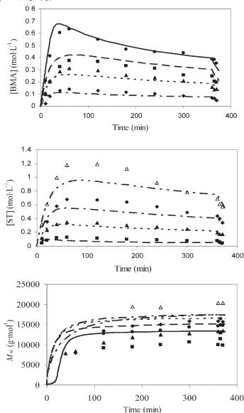
**Figure 5.**[BMA], [ST] and weight-average MW model predictions (lines) compared to experimental results (points): BMA homopolymerization (—, ●); ST homopolymerization (— - - -, △); BMA/ST 75/25 copolymerization (— --, ■); BMA/ST 50/50 copolymerization (- - -, ▲); BMA/ST 25/75 (— - -, ◆).
